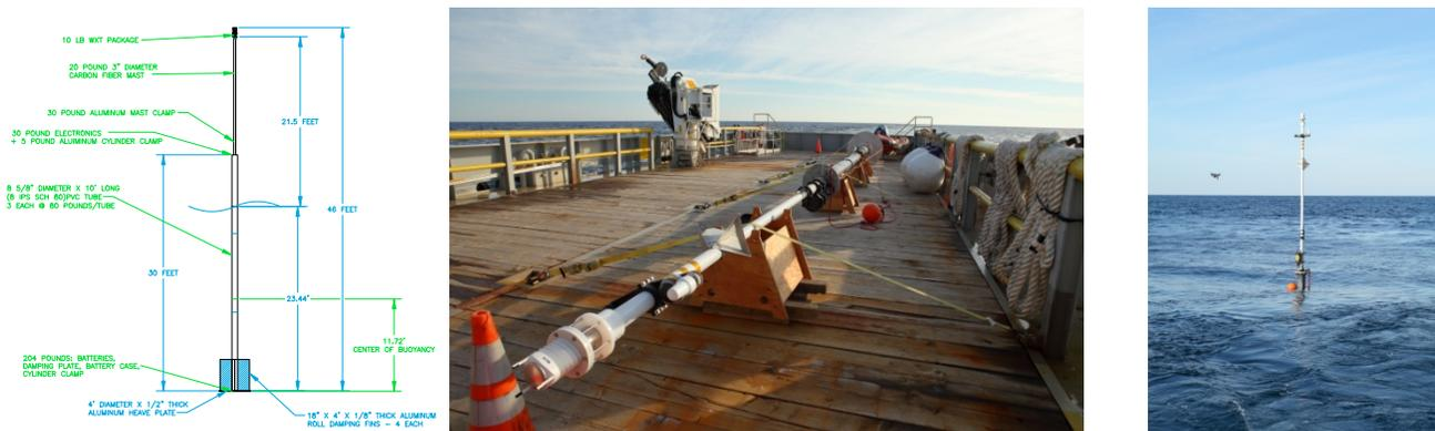
Figure 2. Schematic drawing of the first X-Spar prototype instrument and photographs of it on deck and deployed during a short sea trial.
