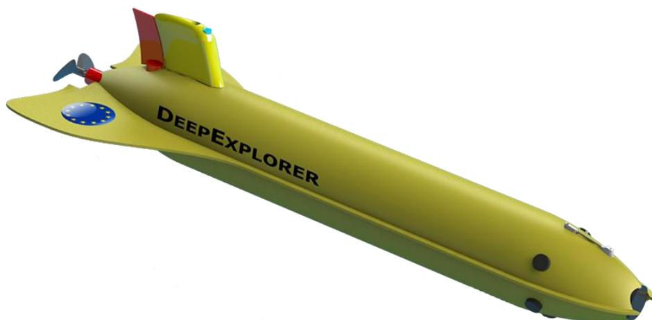
The vehicle design is based upon the Sea Explorer with interchangeable payloads. Battery power is initially expected to be rechargeable lithium ion with primary batteries as an option. Endurance will be of the order of several weeks, dependent on payload. Two vehicles are being designed, the Deep Explorer rated to 2400m and the Ultra-deep Explorer rated to 5000m.
